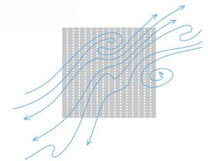
The Pellicle conforms naturally to your contours. It minimises uncomfortable pressure points by properly distributing your weight over the seat and back, away from your spine and the backs of your thighs. Your skin temperature increases up to 12 degrees Fahrenheit (6.7 degrees centigrade) when you sit for 30 minutes in a traditional foam-and-fabric chair. With the Aeron chair, air flows through the Pellicle to prevent heat build-up and allow moisture to dissipate.
