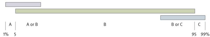
Aeron's B-size chair fits the 5th percentile female to the 95th percentile male. With its A and C sizes, Aeron is the only work chair that also optimises fit for the small and large people toward the ends of the anthropometric bell curve. The sizing accommodates personal preference as well. For many people, either an A or B or a B or C is the appropriate chair size.
