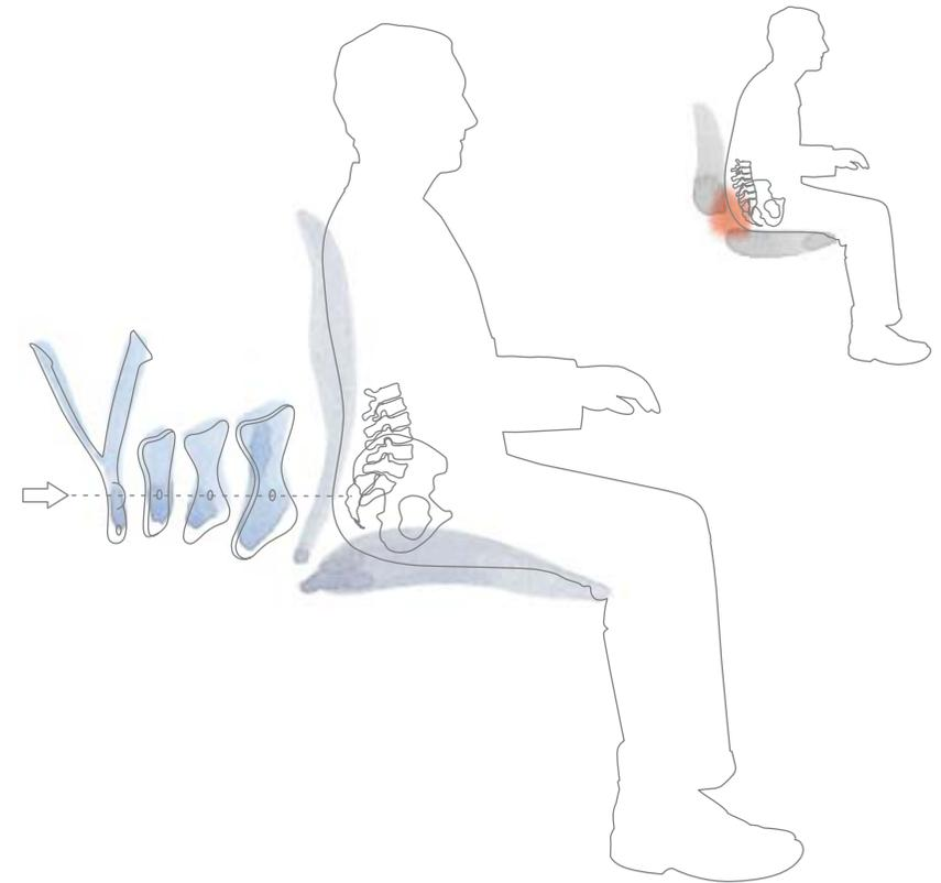
When you sit upright and forward at a computer, there's void between the base of the backrest and your lower back. When that area is unsupported, your hips tend to rotate back and your spine loses its healthful S-shape. In other words, you slouch. PostureFit addresses this root cause of poor posture by filling the void and supporting your lower spine. In addition you can adjust PostureFit to provide the most comfortable level of support.
